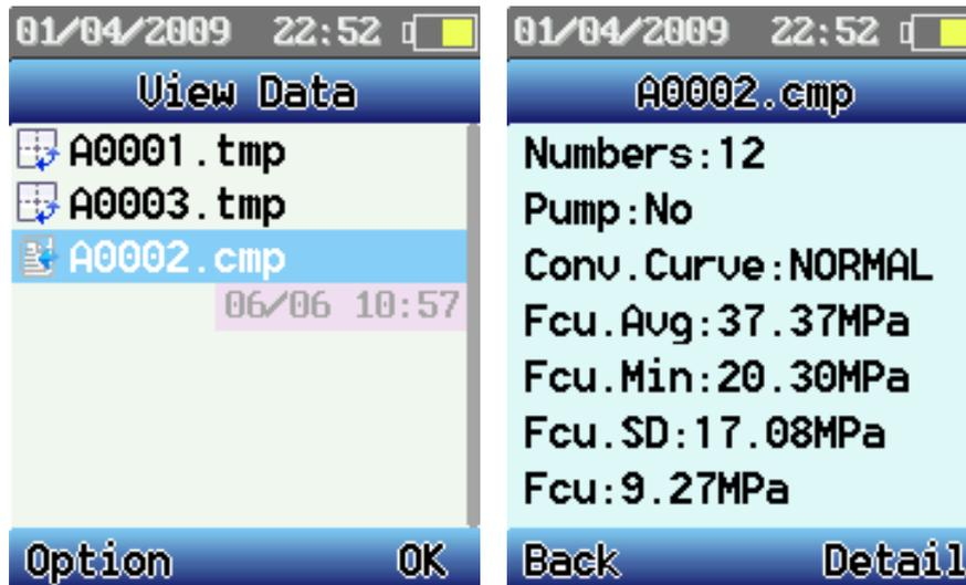
choose one component, **OK** key to show component data, **Detail** key to check details.
