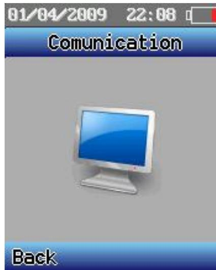
This function is that take the instrument memory as a virtual USB disk, computer can upload or download components data and measuring curve data, do not have to install driver.
