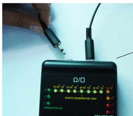
When the cables have been plugged in the appropriate socket, the parallel probes under the meter disengage.
