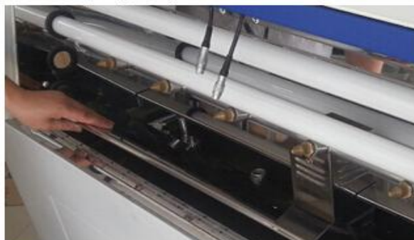
Take out the water proof shield and clean the room
