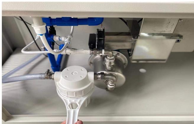
**Picture 29: Replace BUUV filter element**
