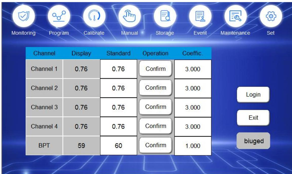
**Picture 33: Calibrate BUV Black Panel Temperature**
