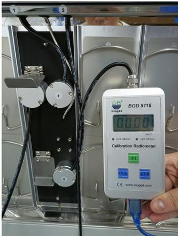
Put the radiometer sensor near that sensor needed to be calibrated
