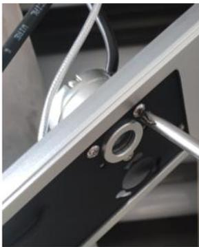
① Loosen the sensor fixing screw and take out the sensor
