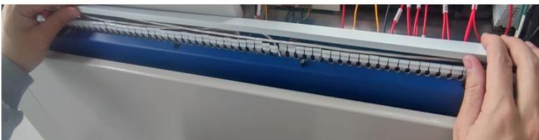
④ Open the wire slot cover and take out the sensor wire
