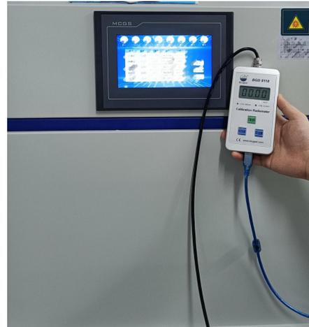
Close BUV front door, compare the value read from radiometer and BUV showing value.
