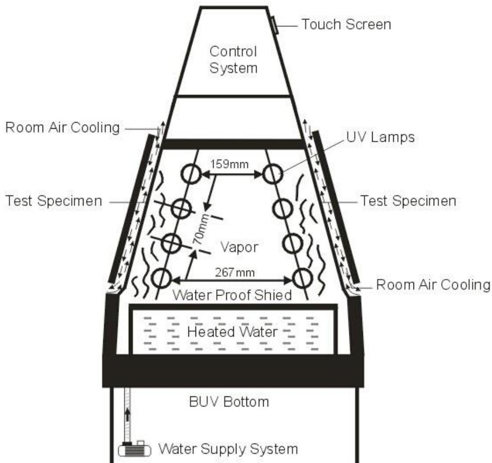
**Picture 1: BUUV Test principle**
