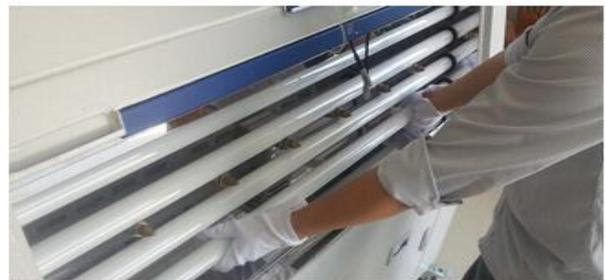
**2- Hold two ends to rotate lamps**
