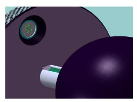
Universal type hammer: Rotating the back cover, change the energy which need to test, then do the test same as the Single Type Hammer.
