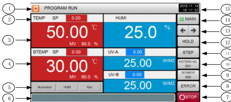
[Figure 3-7] PROGRAM Operation--The 1<sup>st</sup> RUN screen
