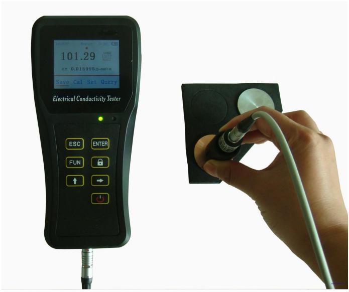
FD102 is a kind of eddy current electrical conductivity meter, which is designed for quick & convenient measurement of material property, such as material separate, quality control, material state check and so on. It uses the electromagnetism testing principle. Testing objects focus on non-ferromagnetic material.
