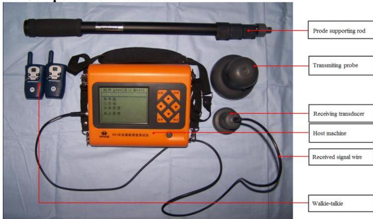
Diagram 1-2 Component of Instrument
