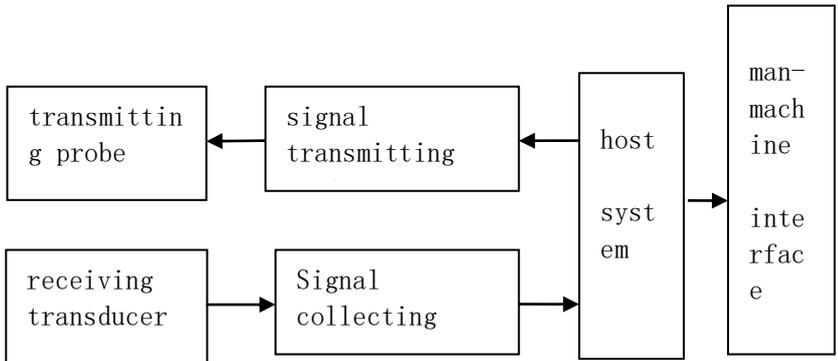
Diagram 1-1 Operating Principle of the non metal plate thickness admeasuring apparatus
