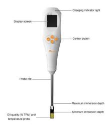
Figure 1 Front View of Cooking Oil Tester
