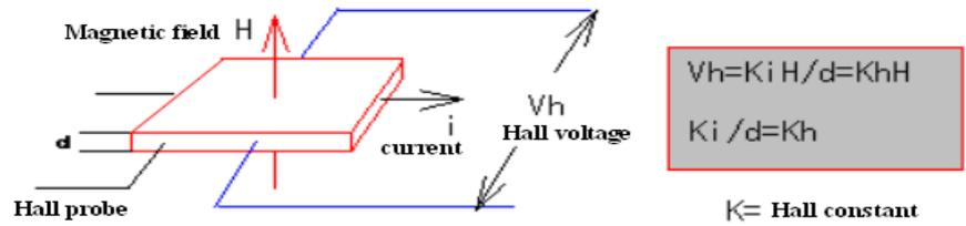
When placing the semiconductor carrying current in the magnetic field axial to the current direction, the semiconductor will generate transverse galvanomagnetic phenomenon, namely generate electromotive force in the direction axial to the magnetic field and current, which is Hall Effect. Hall Effect can be explained with classical galvanomagnetic theory. Generally, Hall voltage  $U_H$  is expressed as:
